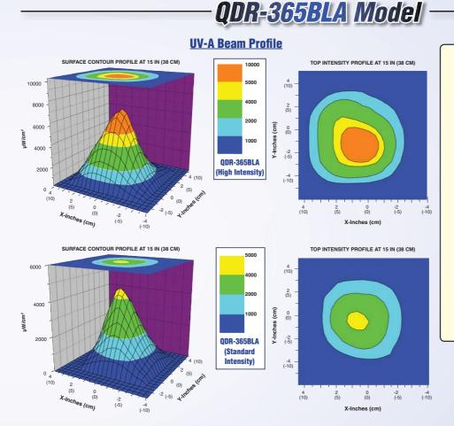
The **QDR-365BLA** is equipped with a faceplate with <u>integral</u> <u>black light</u> filters that reduce the output of wavelengths longer than 400 nm. When in the *high intensity* mode, the lamp provides a nominal steady-state UV-A intensity of *7,000 µW/cm*<sup>2</sup> at 15 inches (38 cm).
